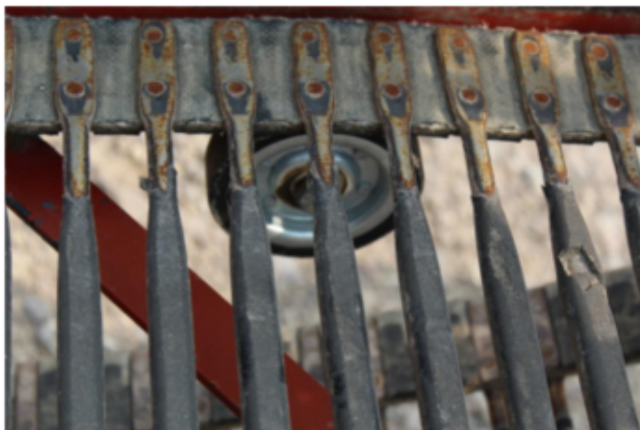
Photo 5. Replace worn padding on chain conveyors. Exposed metal on the chains indicates that the padding is no longer effectively cushioning impacts. The ends of conveyors where they contact rollers are common places for excessive wear.
