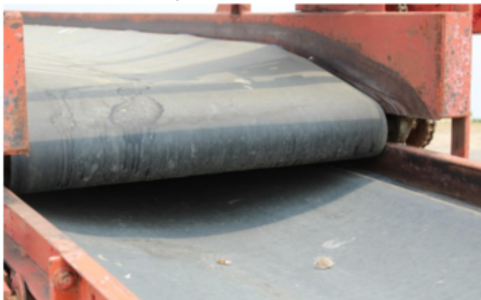
Photo 6. Cleaning equipment before harvesting the new crop is important to minimize disease carryover from one season to the next. Diseases such as bacterial ring rot can survive as dried slime on metal and other surfaces for more than a year. See http://www.cals.uidaho.edu/edComm/pdf/CIS/CIS1180.pdf for more information on cleaning equipment and storages.
