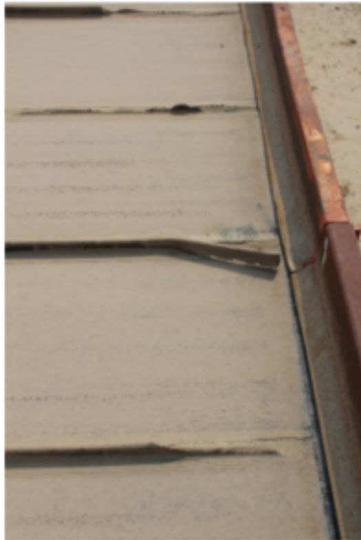
Photo 1. Worn flights should be replaced to properly carry potatoes up conveyors. These flights minimize rollback and bruising of potatoes.
