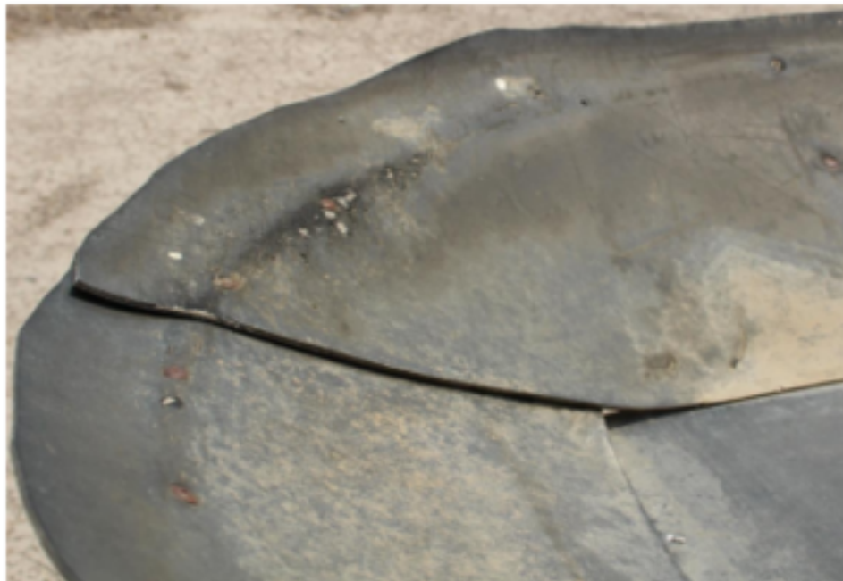
Photo 2. Wear on stinger baskets exposes metal surfaces for potatoes to hit and easily become damaged. It takes less force to bruise potatoes if they are hitting metal compared to belting or other cushioning materials (See figure 1). Replace all worn padding before starting to harvest the new crop.
