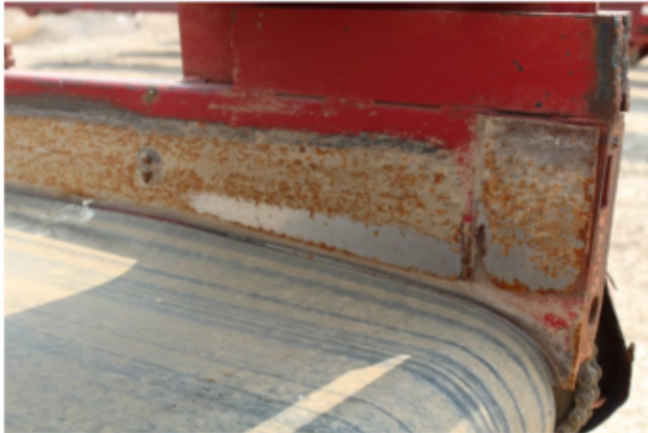
Photo 4. Noticed how shiny and worn down the metal is on the side wall in this photograph? That is from potatoes hitting and rubbing against the metal. Look for areas throughout your operation where you see shiny metal and consider adding padding to minimize the impact on potatoes.
