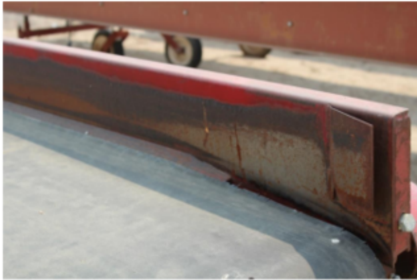
Photo 3. Don't forget to pad sidewalls and replace worn padding to avoid potatoes hitting bare metal.
