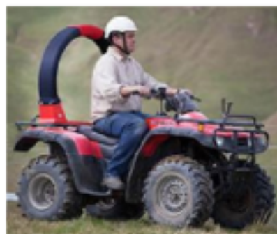
ATV with ROPS and proper personal protective equipment (PPE) (Source: www.cerenti.com/learningpaper/REDUCING-ALL-TERRAIN-VEHICLE-INJURIES-(ATVs)-AND-Backhoes-for-rentals-to-reduce-accidents-if-you-own-one-By-Steve-Tighe/ )
